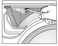
Use a bottle brush to remove any detergent residue and lime deposits from the jets inside the detergent drawer.
